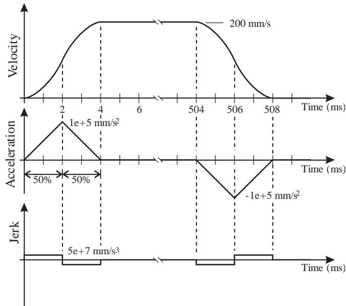
**Figure 3.13.** Motion profiles for S-curve velocity profile with Accel Jerk and Decel Jerk 100% of Time.
