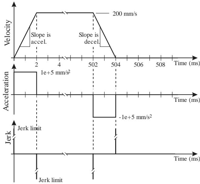
**Figure 3.12.** Motion profiles for trapezoidal velocity profile.
