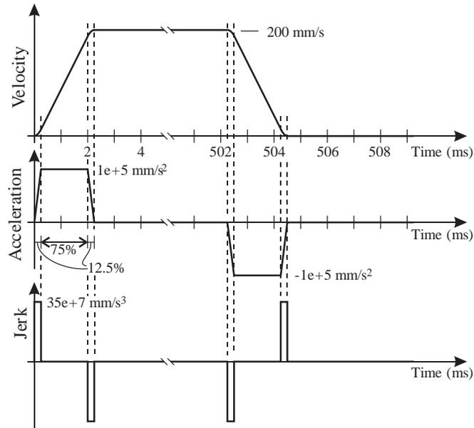
**Figure 3.14.** Motion profiles for S-curve velocity profile with Accel Jerk and Decel Jerk 25% of Time.
